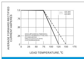
Fig.1 FORWARD CURRENT DERATING CURVE
