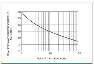
Fig. 2 MAXIMUM NON-REPETITIVEPEAKFORWARD SURGE CURRENT
