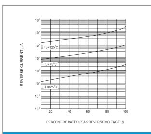
Fig.3 TYPICAL REVERSE CHARACTERISTIC
