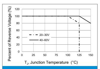
**Fig.5 Operating Temperature Derating Curve**
