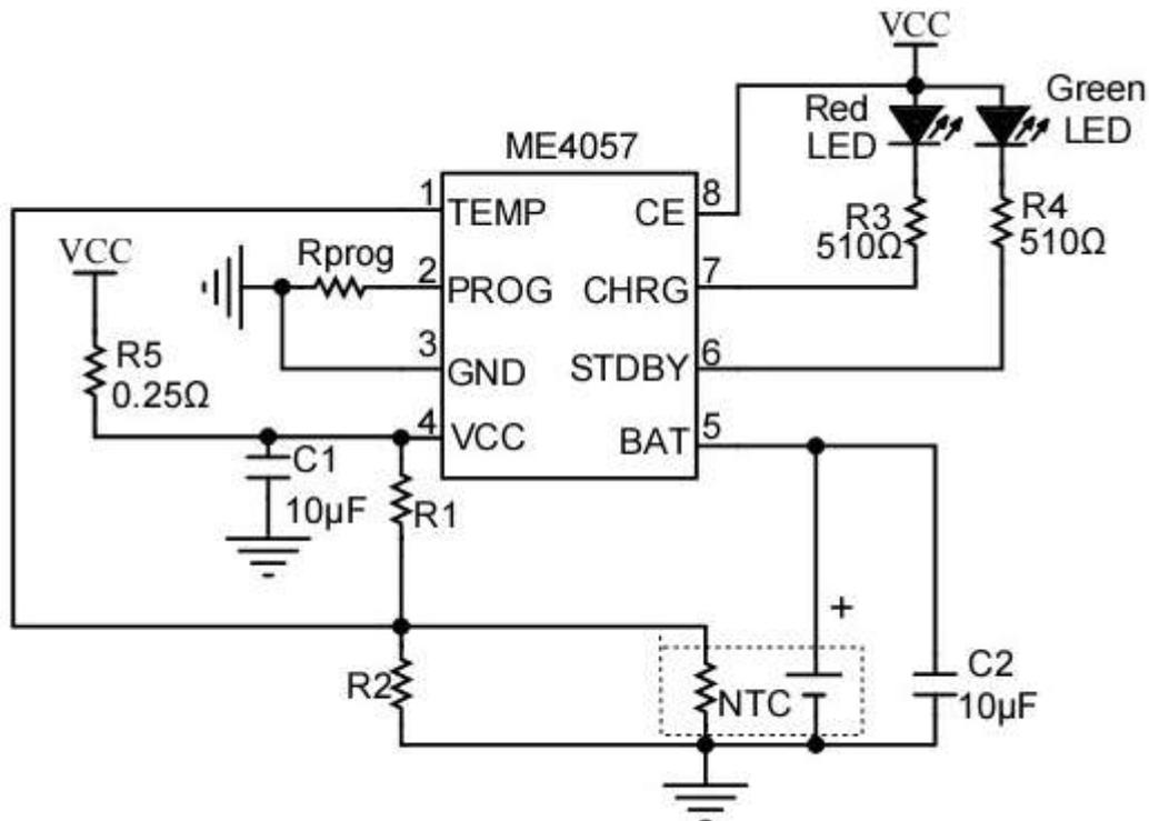
2. Suitable for the application of USB power and the charge of wall adapter
