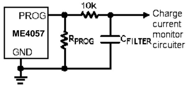
Fig.2 Isolating with capacitive load on PROG Pin
