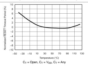
Figure 4. Normalized RESET Timeout Period vs Temperature
