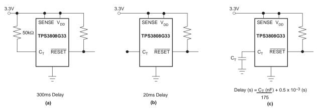
Figure 10. Configuration Used to Set the RESET Delay Time
