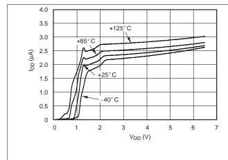
Figure 2. Supply Current vs Supply Voltage
