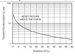
Figure 5. Maximum Transient Duration at Sense vs Sense
