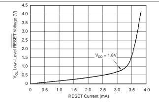
Figure 7. Low-Level  $\overline{\text{RESET}}$  Voltage vs  $\overline{\text{RESET}}$  Current
