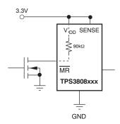
Figure 12. Using an External MOSFET to Minimize I<sub>DD</sub> When MR Signal Does Not Go to V<sub>DD</sub>
