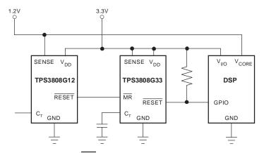
Figure 11. Using MR to Monitor Multiple System Voltages
