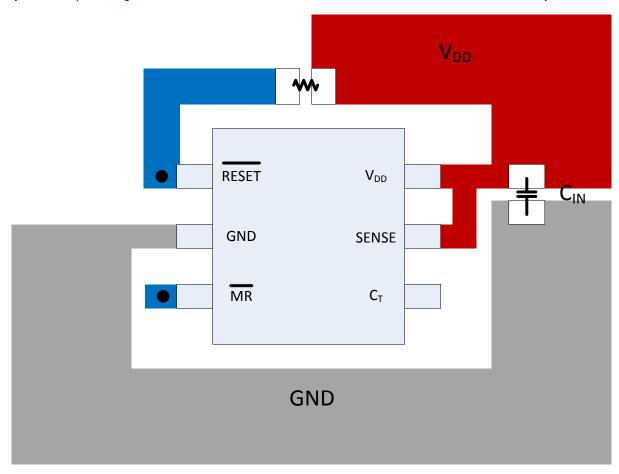
VIAS USED TO CONNECT PINS FOR APPLICATION SPECIFIC CONNECTIONS
