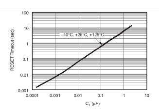
Figure 3. RESET Timeout Period vs C<sub>T</sub>
