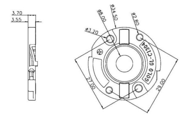
Chip-on-Board (COB) LED Array Holders: CREE LED
