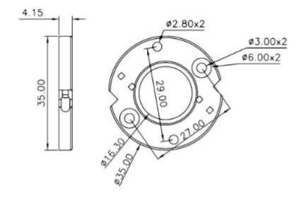
Chip-on-Board (COB) LED Array Holders: CREE LED
