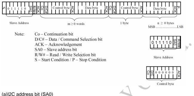
The slave address is following the start condition for recognition use. The slave address is either "b0111100" or "b0111101" by changing the SA0 to LOW or HIGH (D/C pin acts as SA0).
