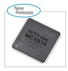
MCX514 is 4-axis Motion Control IC which connects to CPU with 8/16-bit or I<sup>2</sup>C serial interface bus and can control either a stepper motor driver or pulse type servo driver for position and speed.
