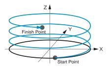
In addition to linear and circular, helical interpolation can be executed which drives another axis synchronous with circular interpolation on X,Y surface. Example of multiple rotation of helical interpolation in the above figure.
