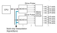
Multi-axis linear interpolation with 5 or more axes can be executed by connecting multiple MCX514.
