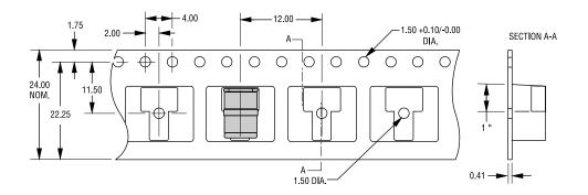
TOLERANCES: ±0.13 UNLESS OTHERWISE SPECIFIED DIMENSIONS: MILLIMETERS
