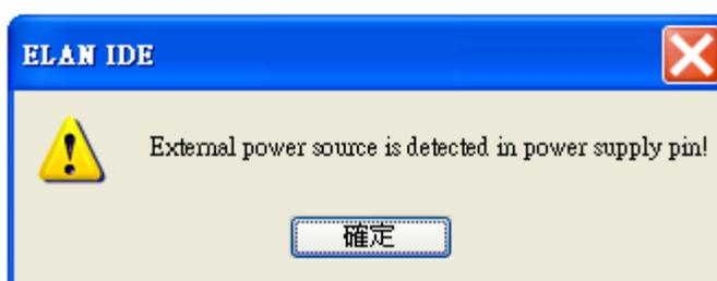
Figure 2-7 External Power Source Error Message
