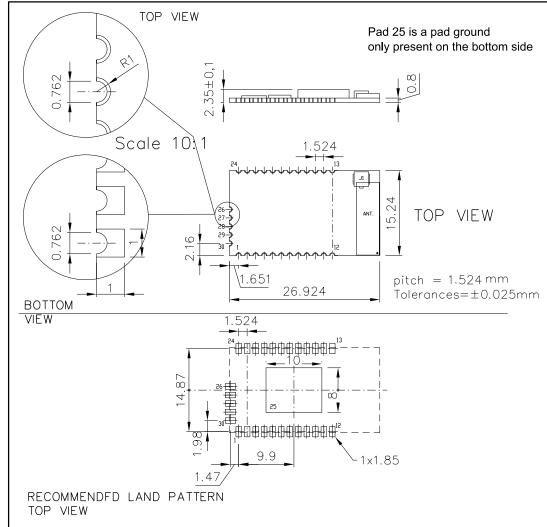
Figure 2: SPWF01SA module footprint
