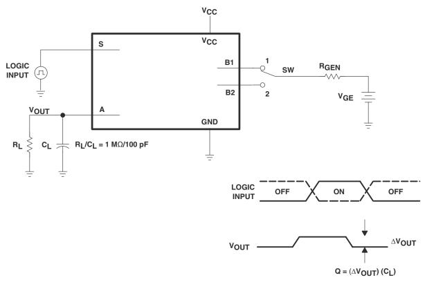
Figure 9. Charge-Injection Test
