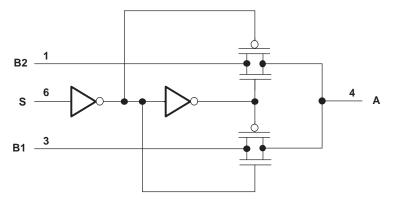
Figure 12. Logic Diagram (Positive Logic)
