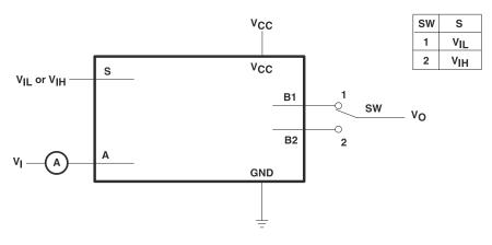
$\begin{array}{l} \mbox{Condition 1: } V_I = \mbox{GND}, \ V_O = V_{CC} \\ \mbox{Condition 2: } V_I = V_{CC}, \ V_O = \mbox{GND} \\ \end{array}$
