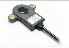
The PST-360 through / hollow shaft position sensors combines three critical design features; 1) through hole where the shaft passes through the sensor, 2) high accuracy absolute position feedback over up to 360°, and 3) a true non-contacting sensing element. Piher's design does not rely on gears or other rotating parts.
