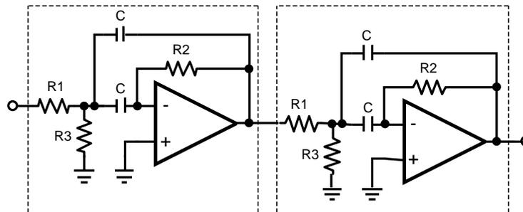
Figure 38. Active Band-Pass Filter Implementation
