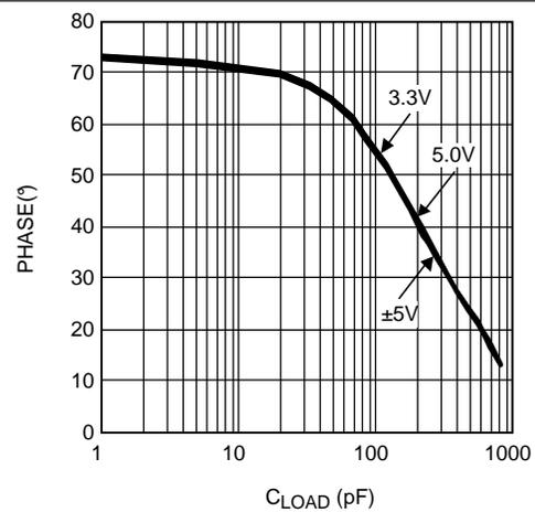
Figure 20. Phase Margin vs  $C_L$
