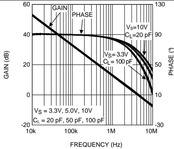
Figure 19. Open-Loop Frequency Response Over Load Conditions
