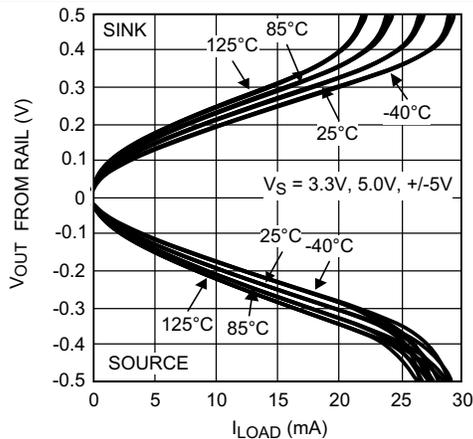
**Figure 17. Output Voltage Swing vs Load Current**
