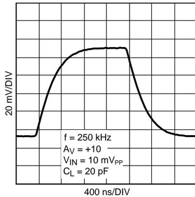
Figure 27. Small Signal Step Response With Gain = 10
