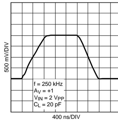
Figure 24. Large Signal Step Response With Gain = 1
