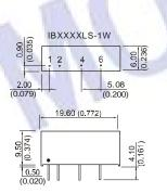
RECOMMENDED FOOTPRINT Top view,grid:2.54\*2.54mm(0.1\*0.1inch), diameter:1.00mm(0.039inch)
