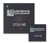
Support for 4 spatial streams with unequal modulation per stream enables up to 600 Mbps PHY data rates and best-in-class performance. Support for Low-Density Parity Check (LDPC) enables efficient error correction coding for superior coverage and improved range.
