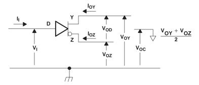
Figure 9. Driver Voltage and Current Definitions
