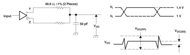
A. All input pulses are supplied by a generator having the following characteristics: t<sub>r</sub> or t<sub>f</sub> ≤ 1 ns, pulse repetition rate (PRR) = 0.5 Mpps, pulse width = 500 ± 10 ns. C<sub>L</sub> includes instrumentation and fixture capacitance within 0.06 mm of the device under test. The measurement of V<sub>OC(PP)</sub> is made on test equipment with a –3dB bandwidth of at least 300 MHz.
