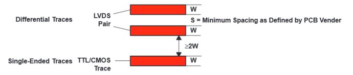
Figure 28. 3-W Rule for Single-Ended and Differential Traces (Top View)
