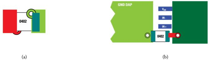
Figure 30. Typical Decoupling Capacitor Layouts
