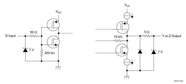
Figure 15. Driver Equivalent Input and Output Schematic Diagrams
