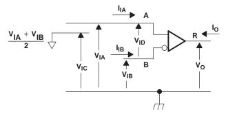
Figure 11. Receiver Voltage and Current Definitions
