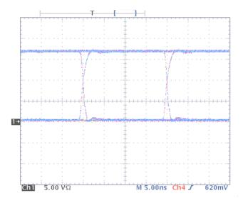
Figure 21. Typical Driver Output Eye Pattern in Point-to-Point System
