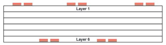
Figure 31. Staggered Trace Layout
