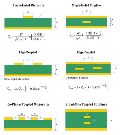
Figure 20. Controlled-Impedance Transmission Lines
