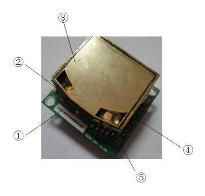
① main board② light source③ air chamber④ contact pin⑤ probe
