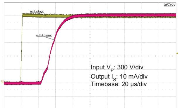
Figure 6: Typical step response (0 to 1500 V)
