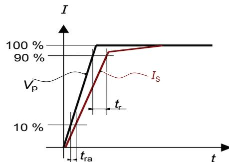
Figure 17: *response time  $t_r$  and reaction time  $t_{ra}$*
