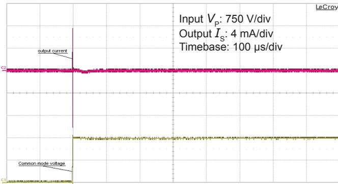
Figure 11: Typical common mode perturbation (1500 V step with 6 kV/μs  $R_M = 100 \Omega$ )
