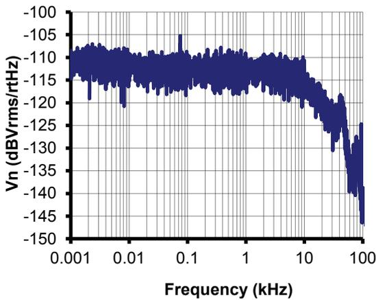
Figure 13: Typical noise voltage density of  $V (R_M)$  with  $R_M = 50 \Omega$
