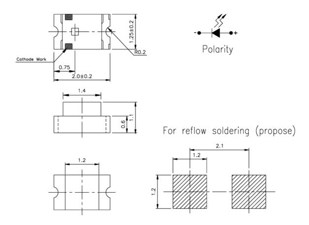
**Note:** The tolerances unless mentioned are  $\pm 0.1$ , unit = mm.
