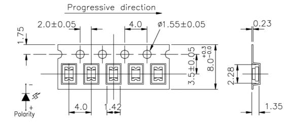
**Note:** The tolerances unless mentioned are  $\pm 0.1$ , unit = mm.
