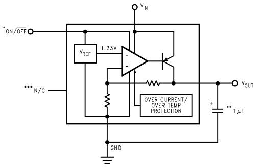
\*ON/OFF input must be actively terminated. Tie to V<sub>IN</sub> if this function is not to be used. \*\*Minimum output capacitance is 1 µF to ensure stability over full load current range. More capacitance provides superior dynamic performance and additional stability margin (see *Output Capacitor Recommendation*). \*\*\*Do not make connections to this pin.
