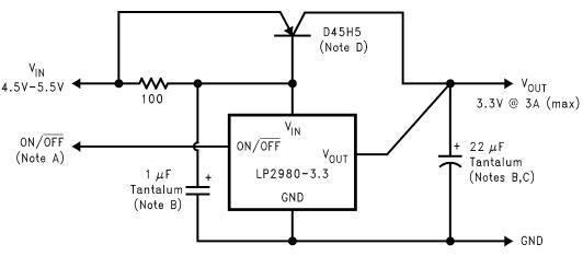
Figure 38. 5 V to 3.3 V at 3-A Converter
