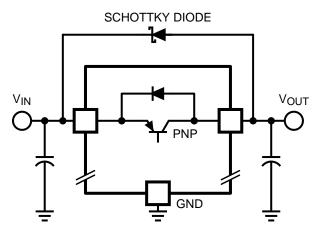
Figure 35. Adding External Schottky Diode Protection
