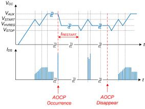
Figure 22. AOCP Waveforms
