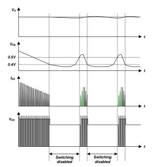
Figure 29. Burst Mode Operation
