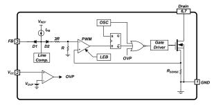
Figure 24. OVP Circuit
