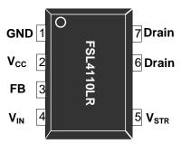
Figure 3. Pin Configuration (Top View)
