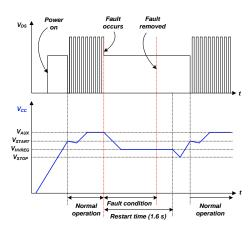
Figure 19. Auto-Restart Protection Waveforms
