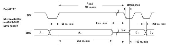
Figure 22. Microcontroller to ADNS-2620 SDIO handoff.
