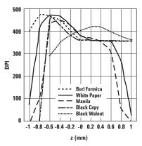
Figure 14. Typical Resolution vs. Z (comparative surfaces)
