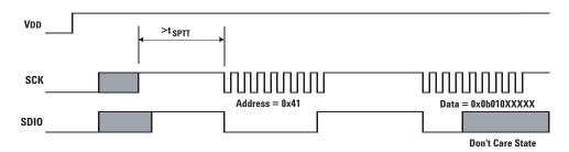
Figure 29. Power-up serial port timer sequence.
