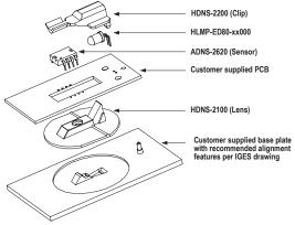
Figure 5. Exploded view drawing.
