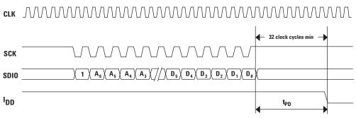
Figure 12. Power-down timing.
