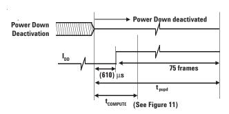
Figure 10. Power up timing mode.
