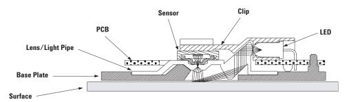
Figure 7. Sectional view of PCB assembly highlighting optical mouse components (optical mouse sensor, clip, lens, LED, PCB and base plate).
