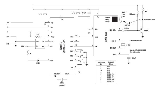
Figure 8. Circuit block diagram for a typical corded optical mouse using an Avago ADNS-2620 optical mouse sensor.
