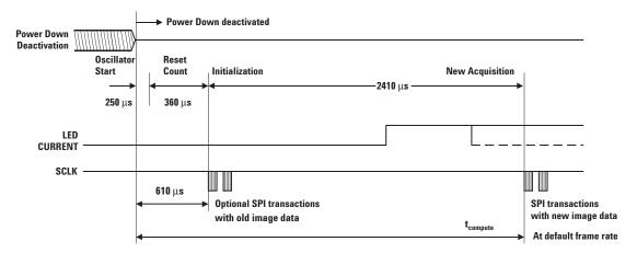
Figure 11. Details of wake-up timing after PD.
