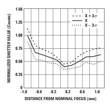
Figure 33. Typical Mean Shutter vs. z (white paper).
