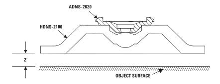
$\label{eq:Figure 9. Distance from lens reference plane to surface. } \\$
