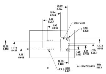
Figure 3. Recommended PCB mechanical cutouts and spacing.
