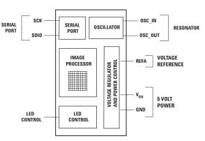
Figure 6. Block diagram of ADNS-2620 optical mouse sensor.
