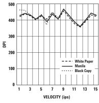
Figure 15. Typical Resolution vs. Velocity @ 1500 fps.
