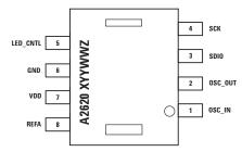
Figure 1. Mechanical drawing: top view.
