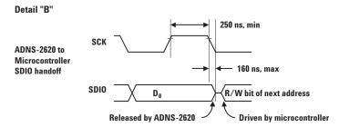
Figure 23. ADNS-2620 to microcontroller SDIO handoff.
