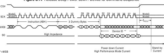
Figure 8.14 Release Deep Power-down / Device ID Command Sequence
