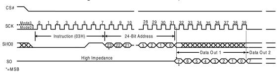
Figure 8.5 Read Data Command Sequence
