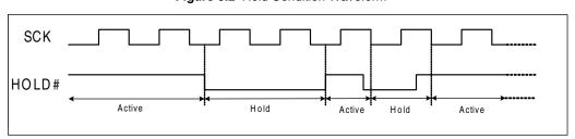
Figure 6.2 Hold Condition Waveform
