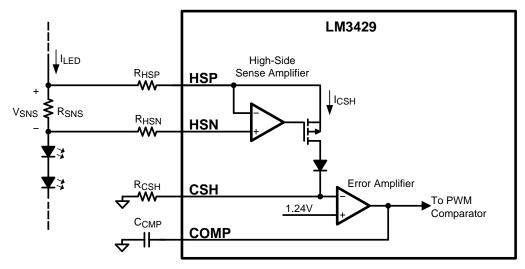
Figure 17. LED Current Sense Circuitry
