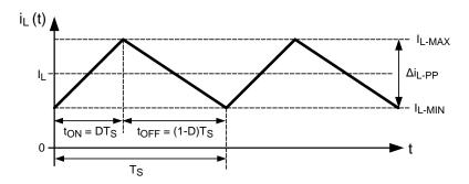
Figure 14. Ideal CCM Regulator Inductor Current i<sub>L</sub>(t)
