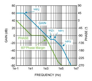
Figure 22. Compensated Loop Gain Frequency Response
