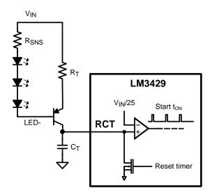
Figure 16. Off-timer Circuitry for Buck Regulators
