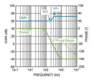
Figure 20. Uncompensated Loop Gain Frequency Response
