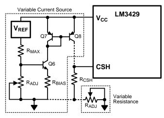
Figure 18. Analog Dimming Circuitry
