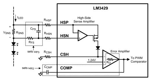
Figure 21. Compensation Circuitry
