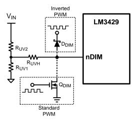
Figure 26. PWM Dimming Circuit
