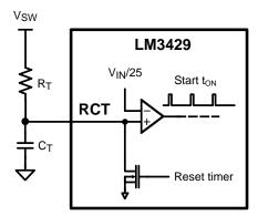
Figure 15. Off-timer Circuitry for Boost and Buck-boost Regulators
