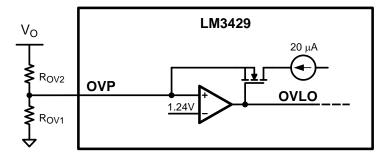
Figure 23. Over-Voltage Protection Circuitry
