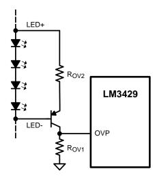
Figure 24. Floating Output OVP Circuitry
