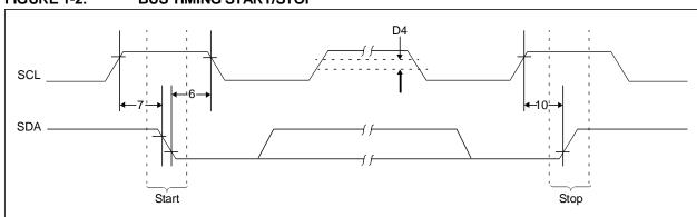
FIGURE 1-2: BUS TIMING START/STOP
