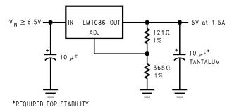
Figure 19. Adjustable at 5 V
