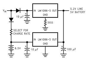
Figure 25. Battery Backup Regulated Supply
