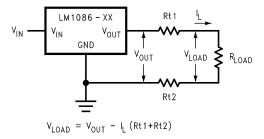
Figure 14. Typical Application Using Fixed Output Regulator
