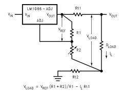
Figure 15. Best Load Regulation Using Adjustable Output Regulator
