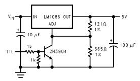
Figure 20. 5-V Regulator with Shutdown
