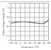
Figure 3. Load Regulation vs Temperature
