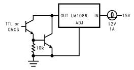
Figure 24. High Current Lamp Driver Protection
