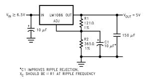
Figure 26. Ripple Rejection Enhancement
