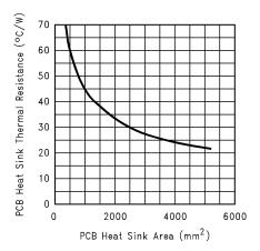
Figure 31. Heat Sink Thermal Resistance vs Area
