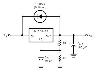
Figure 17. Regulator with Protection Diode
