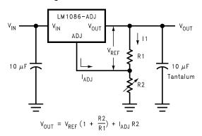
Figure 16. Basic Adjustable Regulator
