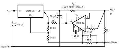
Figure 28. Remote Sensing
