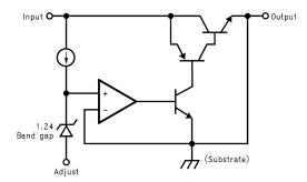
Figure 13. Basic Functional Block Diagram
