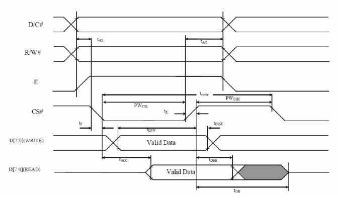
7.3.2 80XX-Series MPU Parallel Interface Timing Characteristics:
