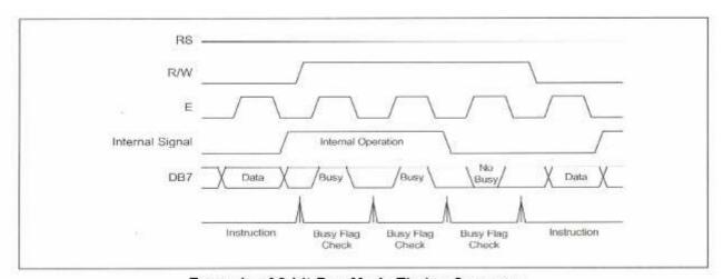
Example of 8-bit Bus Mode Timing Sequence
