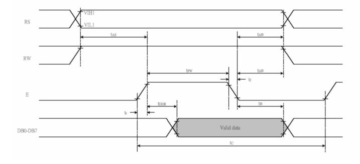
In 6800 interface (TA =  $25^{\circ}$ C, VDD = 2.7V)
