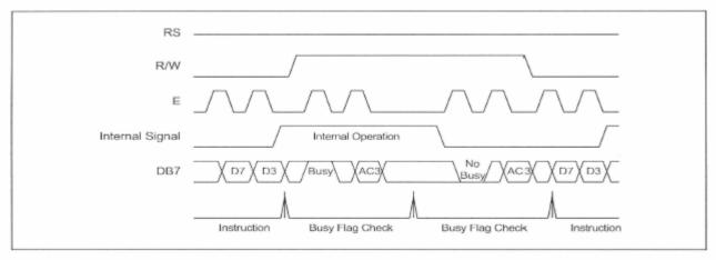
**Example of 4-bit Bus Mode Timing Sequence**
