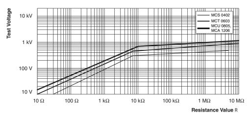
Pulse load rating in accordance with EN 60115-1 clause 4.27; 10  $\mu$ s/700  $\mu$ s; 10 pulses at 1 min intervals; for permissible resistance change  $\pm$  (0.5 % R + 0.05  $\Omega$ )
