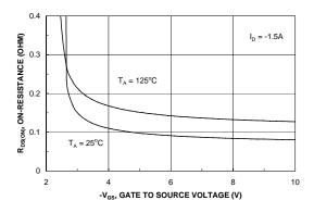
Figure 4. On-Resistance Variation with Gate-to-Source Voltage.
