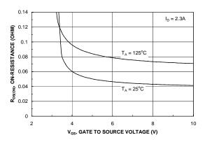
Figure 14. On-Resistance Variation with Gate-to-Source Voltage.
