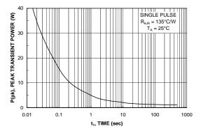
Figure 10. Single Pulse Maximum Power Dissipation.
