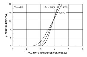
Figure 15. Transfer Characteristics.
