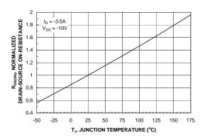
Figure 3. On-Resistance Variation with Temperature.
