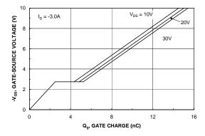
Figure 7. Gate Charge Characteristics.
