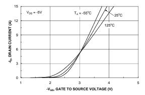
Figure 5. Transfer Characteristics.
