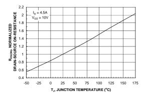
Figure 13. On-Resistance Variation with Temperature.
