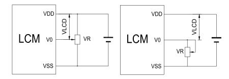
V<sub>DD~</sub>V₀: LCD Driving voltage
