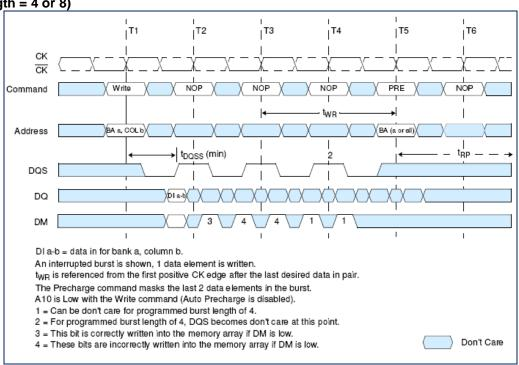
Write to Precharge: Nominal DQSS (2 bit Write), Interrupting (Burst Length = 4 or 8)
