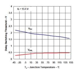
Figure 10. Delay Switching Threshold vs Junction Temperature
