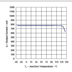
Figure 5. Output Current vs Junction Temperature
