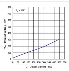
Figure 8. Dropout Voltage vs Output Current
