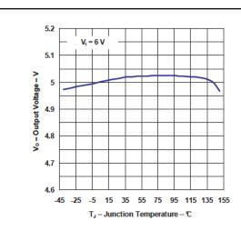
Figure 2. Output Voltage vs Junction Temperature
