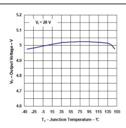
Figure 3. Output Voltage vs Junction Temperature
