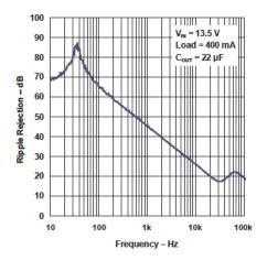
Figure 13. Power-Supply Ripple Rejection vs Frequency
