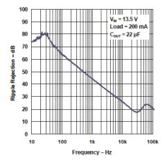
Figure 12. Power-Supply Ripple Rejection vs Frequency
