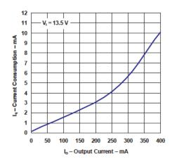
Figure 7. Current Consumption vs Output Current
