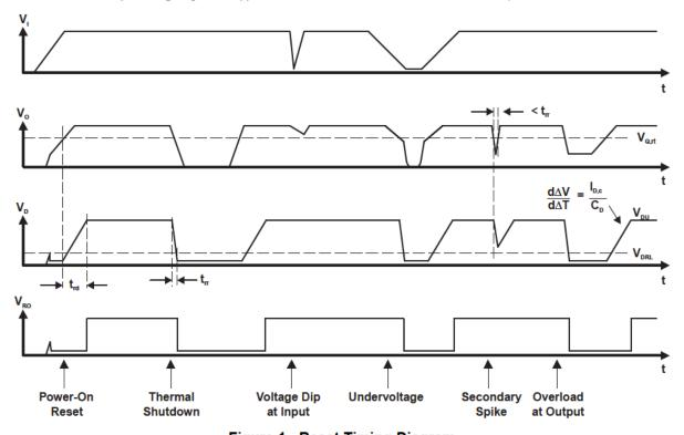
Figure 1. Reset Timing Diagram
