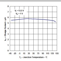
Figure 9. Charge Current vs Junction Temperature
