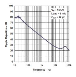
Figure 11. Power-Supply Ripple Rejection vs Frequency
