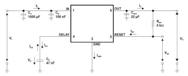
Figure 18. Test Circuit
