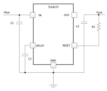
Figure 19. Typical Application Diagram
