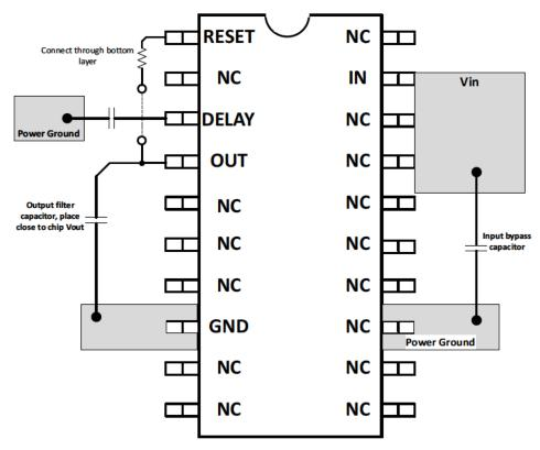
Figure 22. TLE4275-Q1 HTSSOP Layout Design Example
