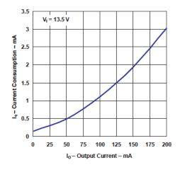
Figure 6. Current Consumption vs Output Current
