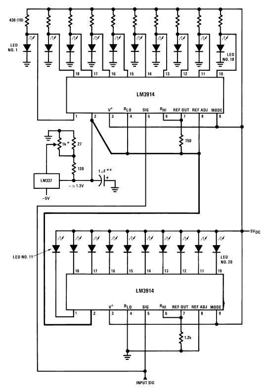
Figure 16. Zero-Center Meter, 20-Segment
