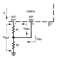
Since the 120µA current (max) from the adjust terminal represents an error term, the reference was designed to minimize changes of this current with V<sup>+</sup> and load changes.
