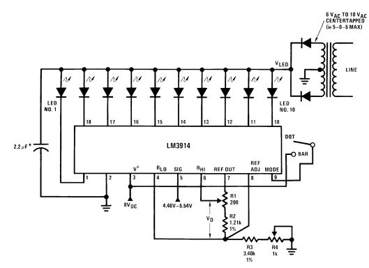
\*This application illustrates that the LED supply needs practically no filtering **Calibration:** With a precision meter between pins 4 and 6 adjust R1 for voltage V<sub>D</sub> of 1.20V. Apply 4.94V to pin 5, and adjust R4 until LED No. 5 just lights. The adjustments are non-interacting.
