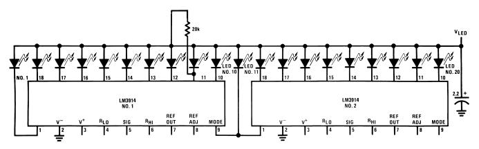
Figure 15. Cascading LM3914s in Dot Mode
