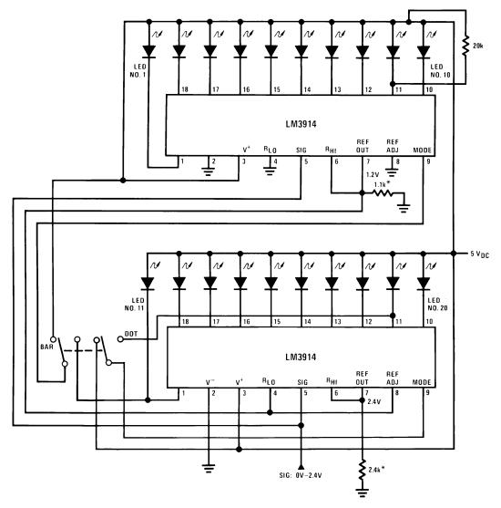
\*The exact wiring arrangement of this schematic shows the need for Mode Select (pin 9) to sense the V<sup>+</sup> voltage exactly as it appears on pin 3. Programs LEDs to 10mA
