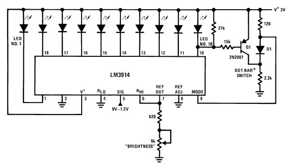
\*The input to the Dot-Bar Switch may be taken from cathodes of other LEDs. Display will change to bar as soon as the LED so selected begins to light.
