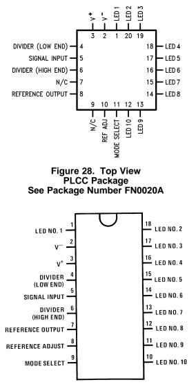
Figure 29. PDIP Package Top View See Package Number NFK0018A
