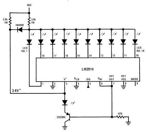
The LED currents are approximately 10mA, and the LM3914 outputs operate in saturation for minimum dissipation. \*This point is partially regulated and decreases in voltage with temperature. Voltage requirements of the LM3914 also decrease with temperature.
