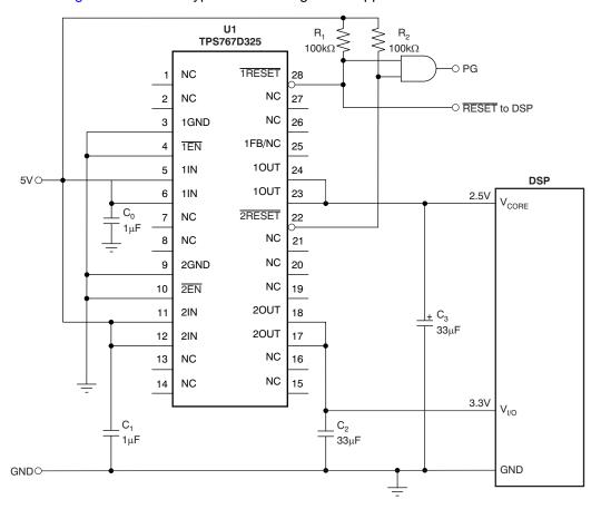
Figure 25. Dual-Voltage DSP Application
