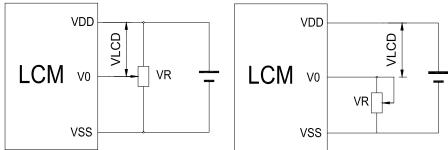
$V_{DD-V_0}$ : LCD Driving voltage VR: 10k~20k
