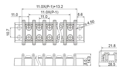
**HOW TO ORDER :** Х Х Х  $\mathbf{P}-$ 1 **Customer Request** Color | Grey 4 Green Series No. NO. of Pole 3 Black DEGSON mm DEGSON ELECTRONICS CO., LTD. (INCH) NAME **DG69-A** THIROANGLE PROJECTION
