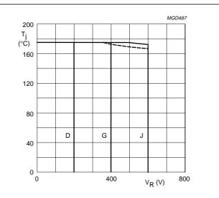
Device mounted as shown in Fig.8. Solid line: Al<sub>2</sub>O<sub>3</sub> printed-circuit board. Dotted line: epoxy printed-circuit board.
