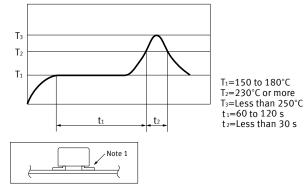
Temperature profile indicates the temperature of the soldered part (Note 1) of terminals on the surface of the PC board, however, for other areas such as the surface of relay case, make a setting so that you do not exceed the recommended conditions.
