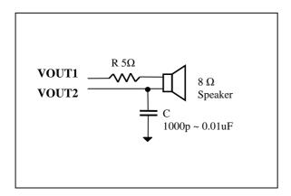
Note: No additional filter connection is needed for  $16\Omega$  speaker.
