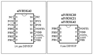
Note: 14 pins and 8 pins packages are available for aIVR3K42
