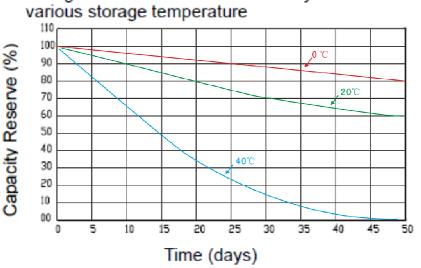
Charge retention curves of Ni-MH cylindrical cell At
