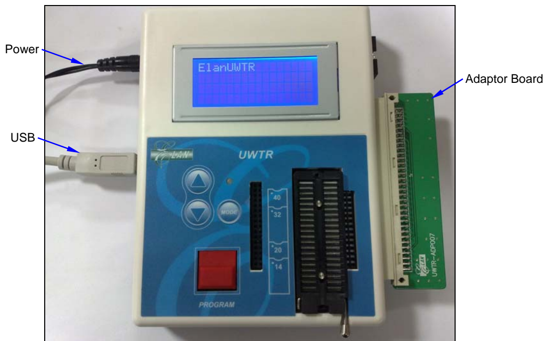
Figure 2-1 Connecting UWTR Writer Assembly to Host Computer
