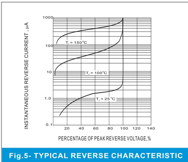
**Fig.5- TYPICAL REVERSE CHARACTERISTIC**
