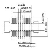
Recommended metal mask pattern Metal mask thickness: When 150 μm (Opening area ratio: 58%)
