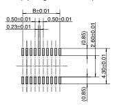
Recommended metal mask pattern Metal mask thickness: When 120 µm (Opening area ratio: 72%)
