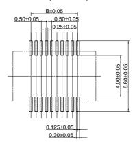
Recommended metal mask pattern Metal mask thickness: When 150 μm (Opening area ratio: 56%)
