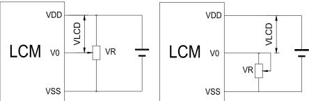
For Module with Normal Temperature Range Fluid V<sub>DD-</sub>V<sub>0</sub>: LCD Driving voltage VR: 10k~20k
