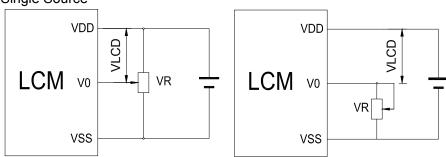
V<sub>DD~</sub>V₀: LCD Driving voltage
