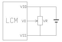
V<sub>DD-</sub>V<sub>0</sub>: LCD Driving voltage VR: 10k~20k
