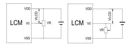
V<sub>DD~</sub>V₀: LCD Driving voltage
