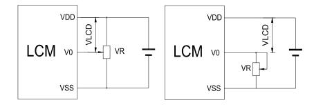
V<sub>DD~</sub>V₀: LCD Driving voltage
