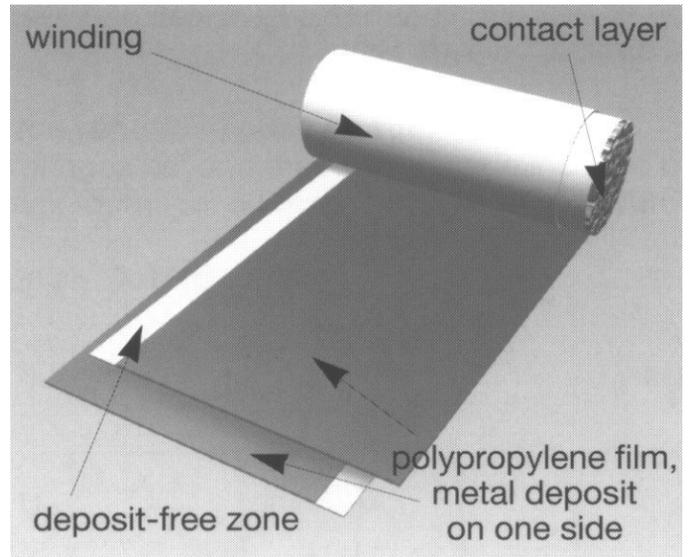
The use of filling materials in capacitors is necessary in order to insulate the capacitor electrodes from oxygen, humidity and other environmental interference. Without such insulation, the metal coating would corrode, an increasing number of partial discharges would occur, the capacitor would lose more and more of its capacitance and suffer increased dielectric losses, and a reduced operating life.
