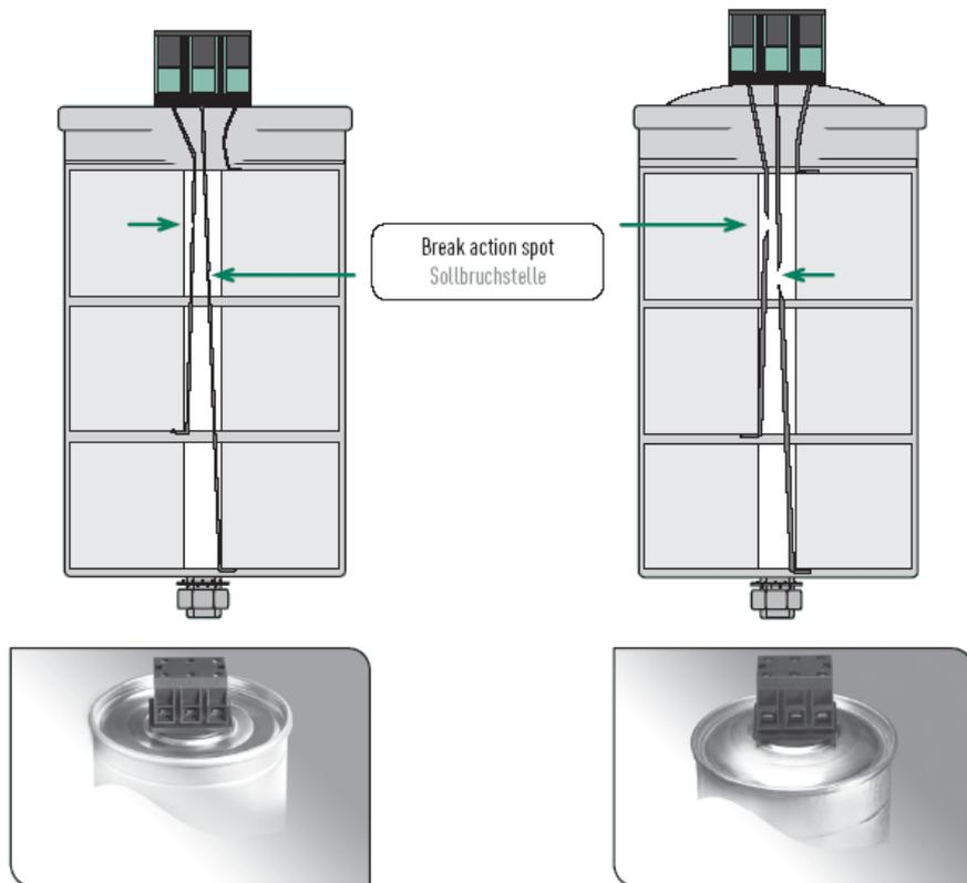
Capacitor before functioning of BAM
